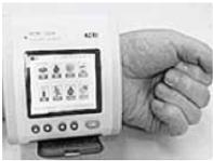
Wrist device for healthcare that monitors blood pressure, body temperature, heart rate.
