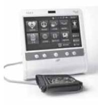
Remote control device for medical treatment that enables telemedicine via a built-in camera and transmits the medical records to the hospital.
